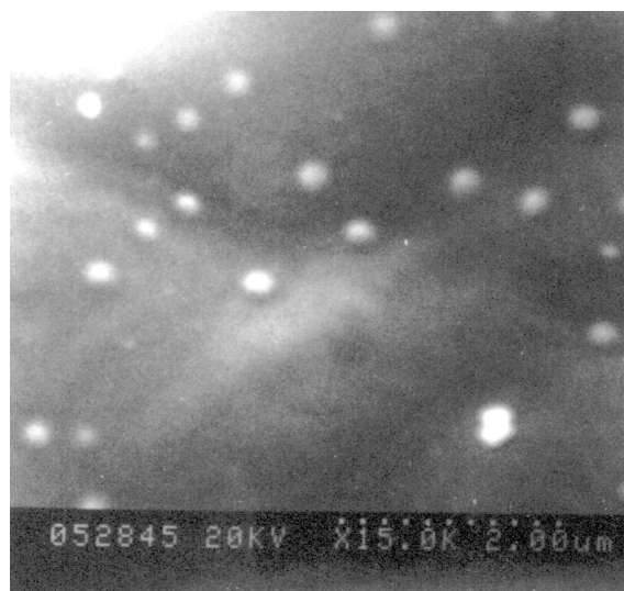
Fig. 3. SEM micrograph of TiO 2 /Ni sample (magnifies to 15000).
